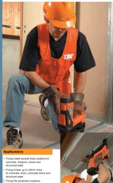
Fixing fire protection systems to steel Fixing angle brackets to concrete brick, block and structural steel Fixing EML to concrete, brick, block and structural steel (using 25mm stee
