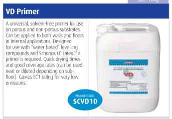
**Application:** As a primer to reduce absorbency of substrates; as a primer to improve adhesion prior to levelling compound application; as a primer to protect against moisture from the levelling compound (see data sheet). Can be applied by brush, roller or spray. Suitable for use on most substrates and can be used over underfloor heating systems. Note: the correct sub-floor preparation must be conducted prior to laying any flooring systems. Consult our technical department for details.
