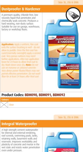
Application: Add to gauging water. To obtain maximum benefit the minimum amount of water should be used in the mix together with an appropriately rich cement to sand aggregate ratio. In application, the mortar must be well compacted to give a dense homogeneous body. Available as either a pink or green liquid.
